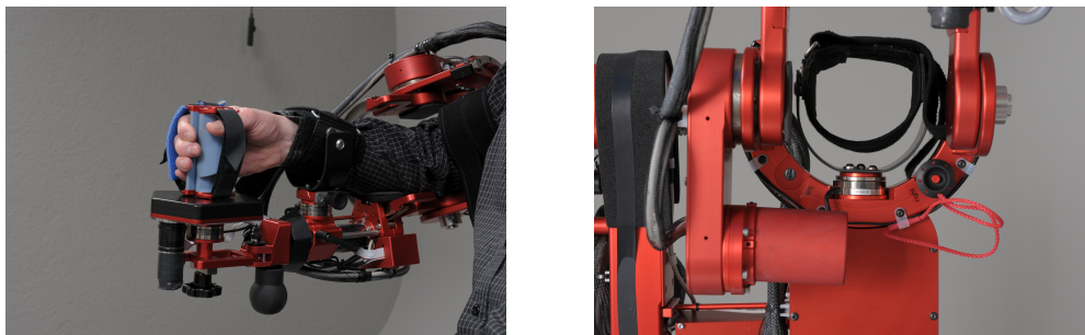
Figure 2.12: Photos of the Force Sensors of the ARMin IV
